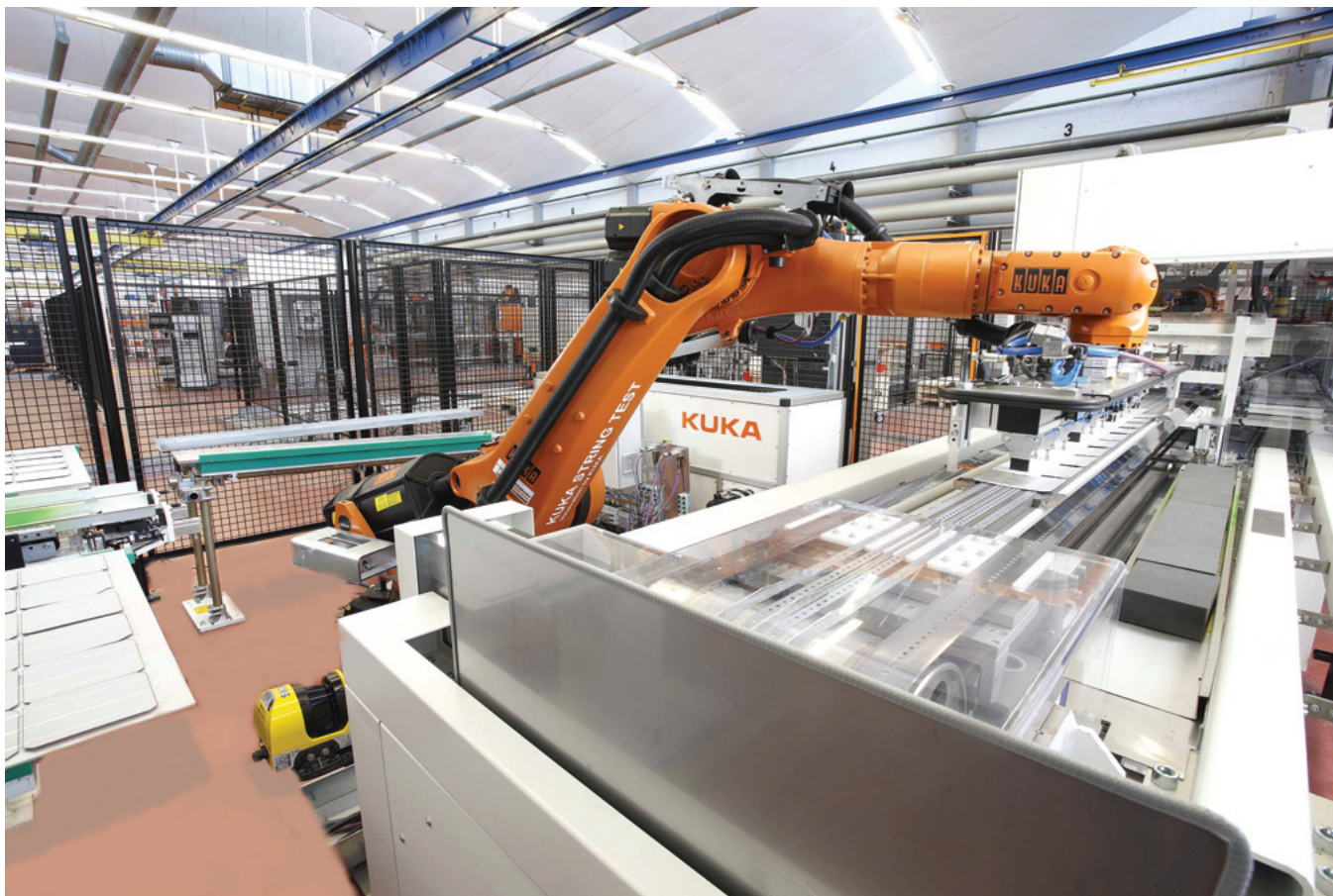
KUKA Systems' automated string testing
