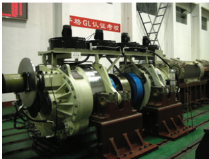
Figure 7: Romax-licensed design for low-noise wind turbine 2 MW gearbox under a vibration test.
