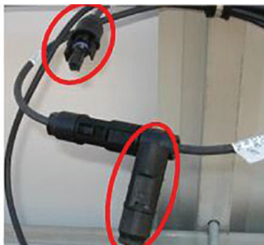
Figure 8: Failed connectors lead to loss of power production.
