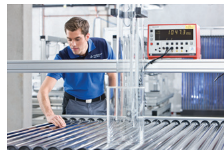
Above: Hail impact testing on a solar collector. Left: Outdoor exposure testing of PV modules. (Photo courtesy of TÜV Rheinland PTL)
