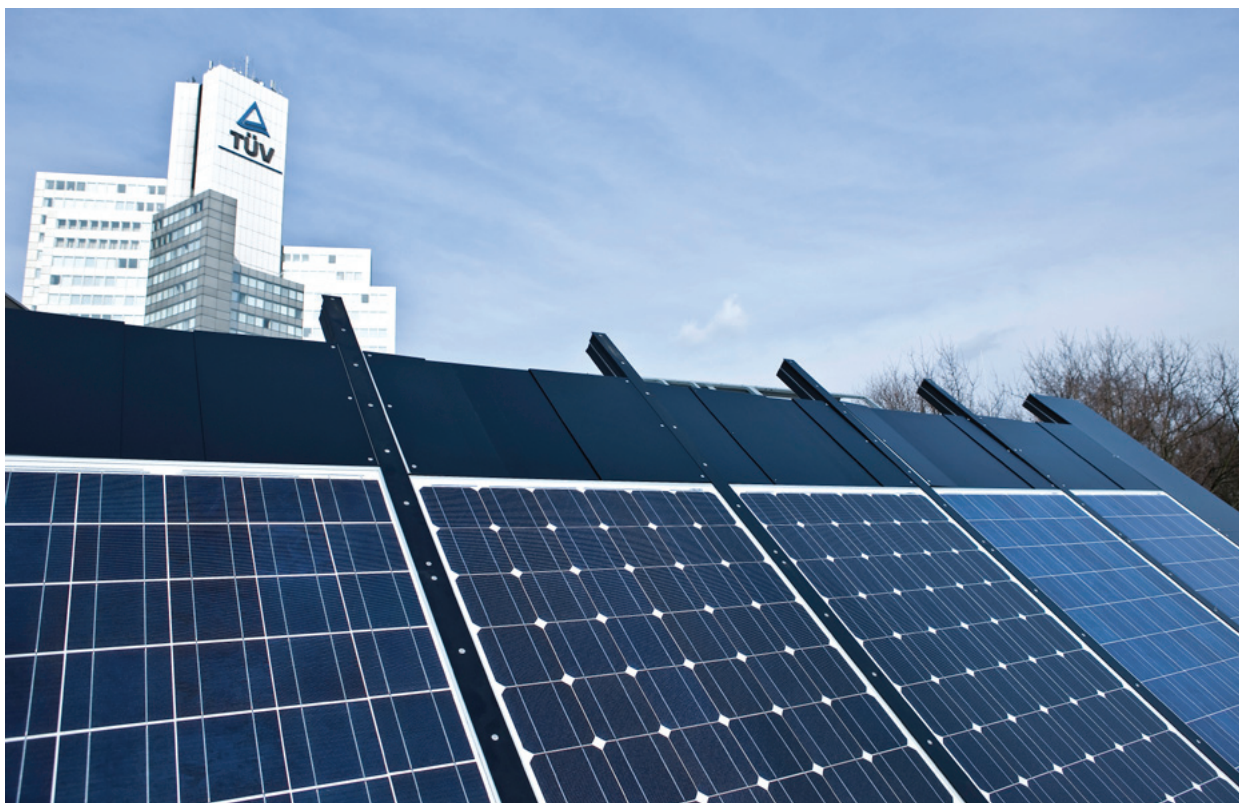
Above: Hail impact testing on a solar collector. Left: Outdoor exposure testing of PV modules. (Photo courtesy of TÜV Rheinland PTL)
