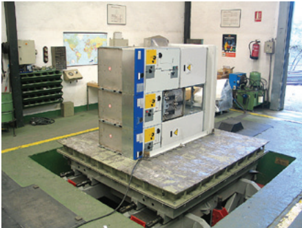
Figure 4. Modular functional units during vibration test.
