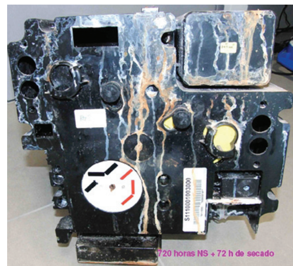
Figure 3. Driving mechanism after a 720-hour salt-spray chamber test. >
