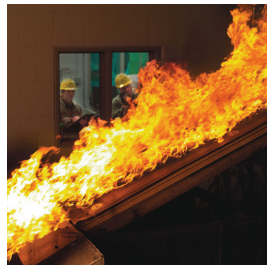
A PV panel being tested to ASTM E 108 fire test at the intended installed slope.
