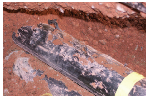
Figure 3: One of seven cable damage locations missed by a VLF test and pinpointed with the offline 50/60Hz PD test.
