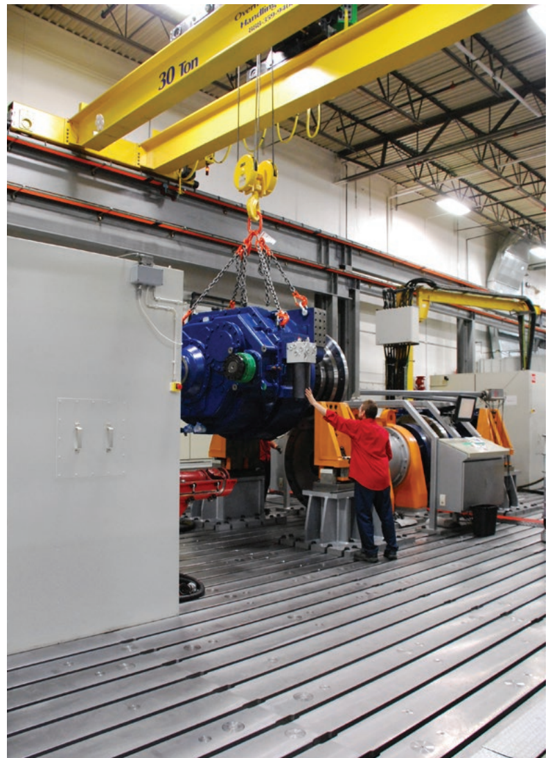
Gearbox being loaded for testing
