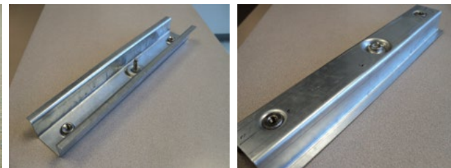
Figure 4. Left image shows the underside view of the hat section, with nuts and stud, while the right image shows the top view
