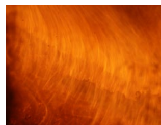
Image 3. Streams of volatile gasses being released from the fuel and rising to the top of the chamber where the combustion process will be complete
