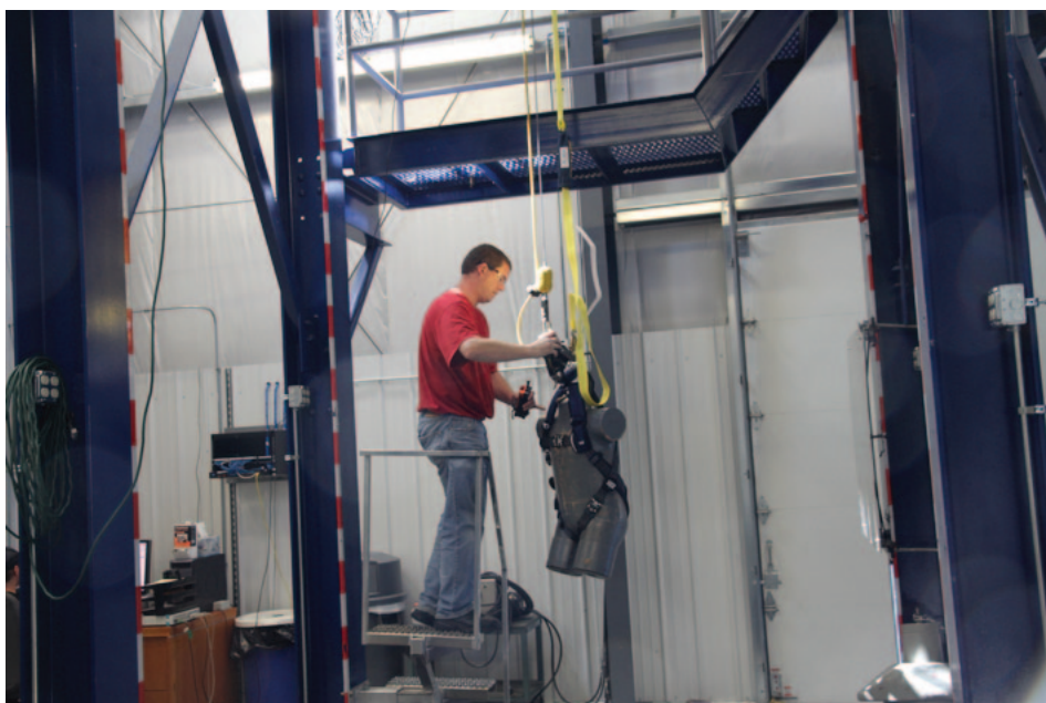
A technician tests a harness with a weighted dummy body. Capital Safety maintains its own testing lab, rather than using an outside facility, in part so that tests are done in a timely manner.
