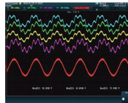
The wave forms of inverter currents from each of the four inverter modules shown. The blue, green, yellow, and magenta oscilloscope tracing show the phase. A distorted currents of each inverter module. The red tracing in the bottom of the picture demonstrate a clean sine wave of harmonically neutralized current delivered into the grid.
