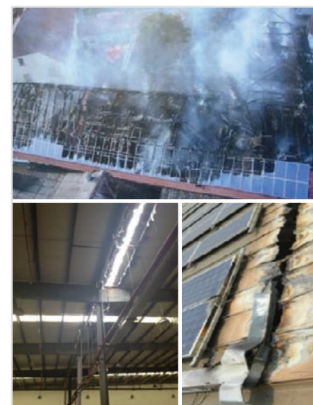
Figure 3. Fire accidents caused by DC arcing
