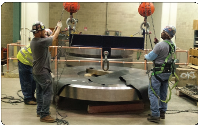
NIST re-assembling the Million Pound Deadweight Testing Machine
