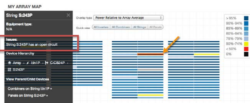
Figure 2. A New Mexico one-megawatt (MW) ground-mount array. The spatial and electrical array map shows the precise location of an open circuit (orange).
