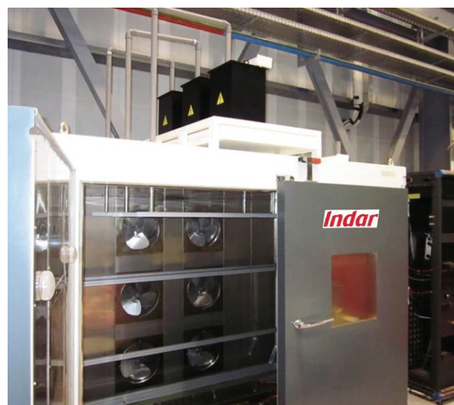
Image 1: Indar Electric 40kV and up to 300C equipment for EIS testing
