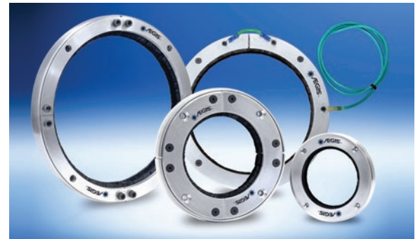
Installed on the 500 HP ventilation fan motor at the Red Trail Energy Ethanol Plant, these rings have 6 rows of conductive microfiber brushes (and millions of shaft contact points) providing the high current-carrying capacity needed for large (500 HP or greater) low-voltage motors, medium-voltage motors, and DC motors (300 HP or greater).
