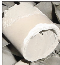
Sulfur cylinder from a flow-line, expelled through a nozzle orifice onto the upper surface of the tower fill.
