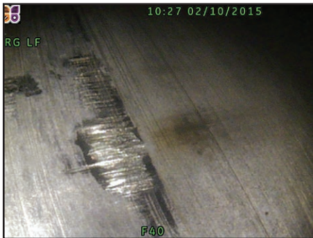
Image 4. Damage observed at the root of a ring gear shortly after turbine commissioning.
