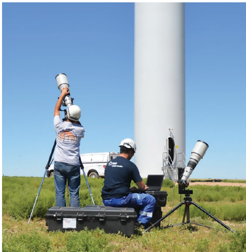
An effective example of a vanguard blade inspection system, a super-zoom camera.
