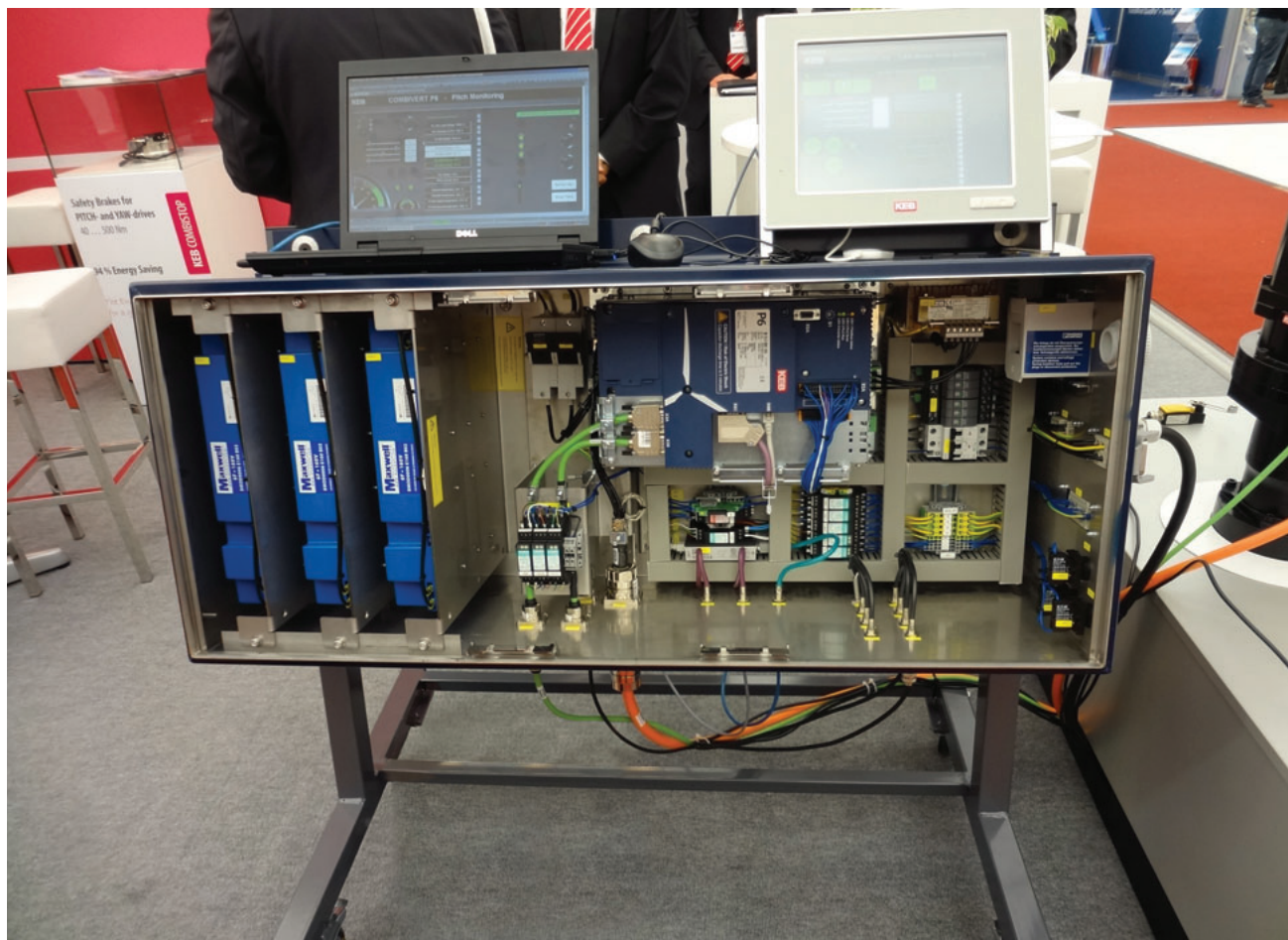
A KEB demonstration of a wind turbine pitch control system, featuring a 160-volt ultracapacitor module (Maxwell Technologies)
