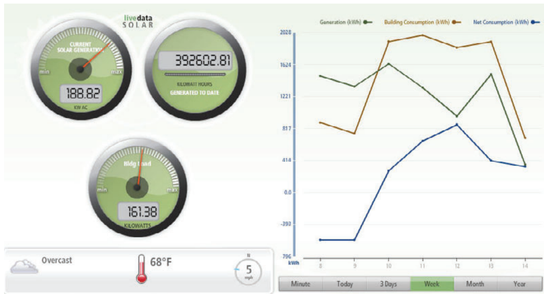
Figure 1. Monitoring interface showing current and historical solar energy production
